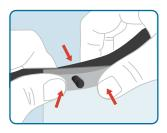
3. Attach visor to headset by snap-fitting each prong to hole (left to right).
